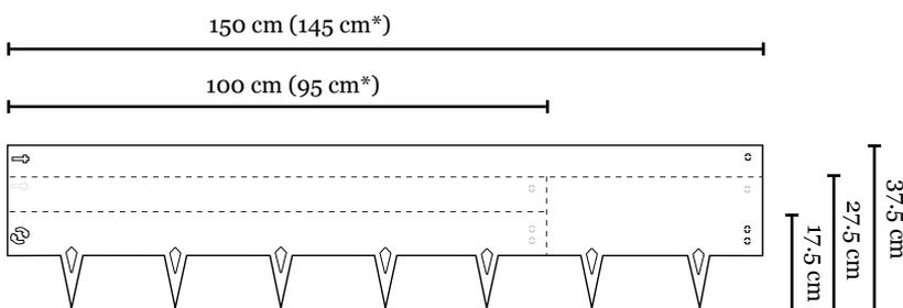
\*working length. To calculate how many segments you need for the total required length you have to edge, divide this length by 0.95 or 1.45.
