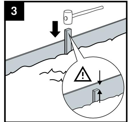
3 Place fixing stakes at 50 cm intervals along the edging. Tap these into the ground using a rubber mallet. Make sure that the fixing stakes protrude a few cm lower than the top edge of the edging. Once installed, the fixing stakes will no longer be visible.
