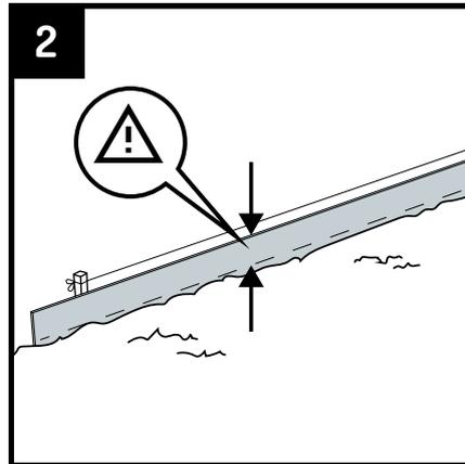
2 Place the edging into the channel. Make sure that at least half of the edging is in the ground. The edging is even more stable when it is inserted deeper into the ground. Cut off any excess length of edging using a hand saw for wood.
