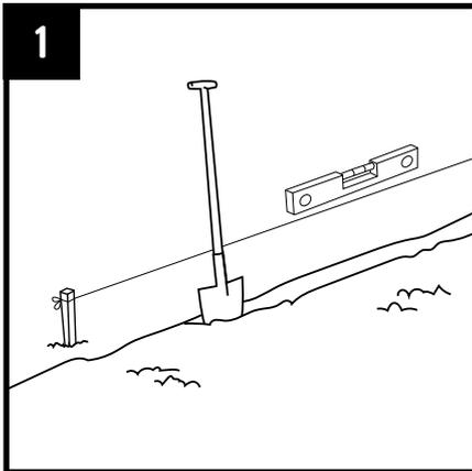
1 Dig a channel. Make sure that at least half of the edging is able to disappear into the channel. For straight edging, mark out the line along which the Multi-Edge ECO is to be installed using twine and pegs.
